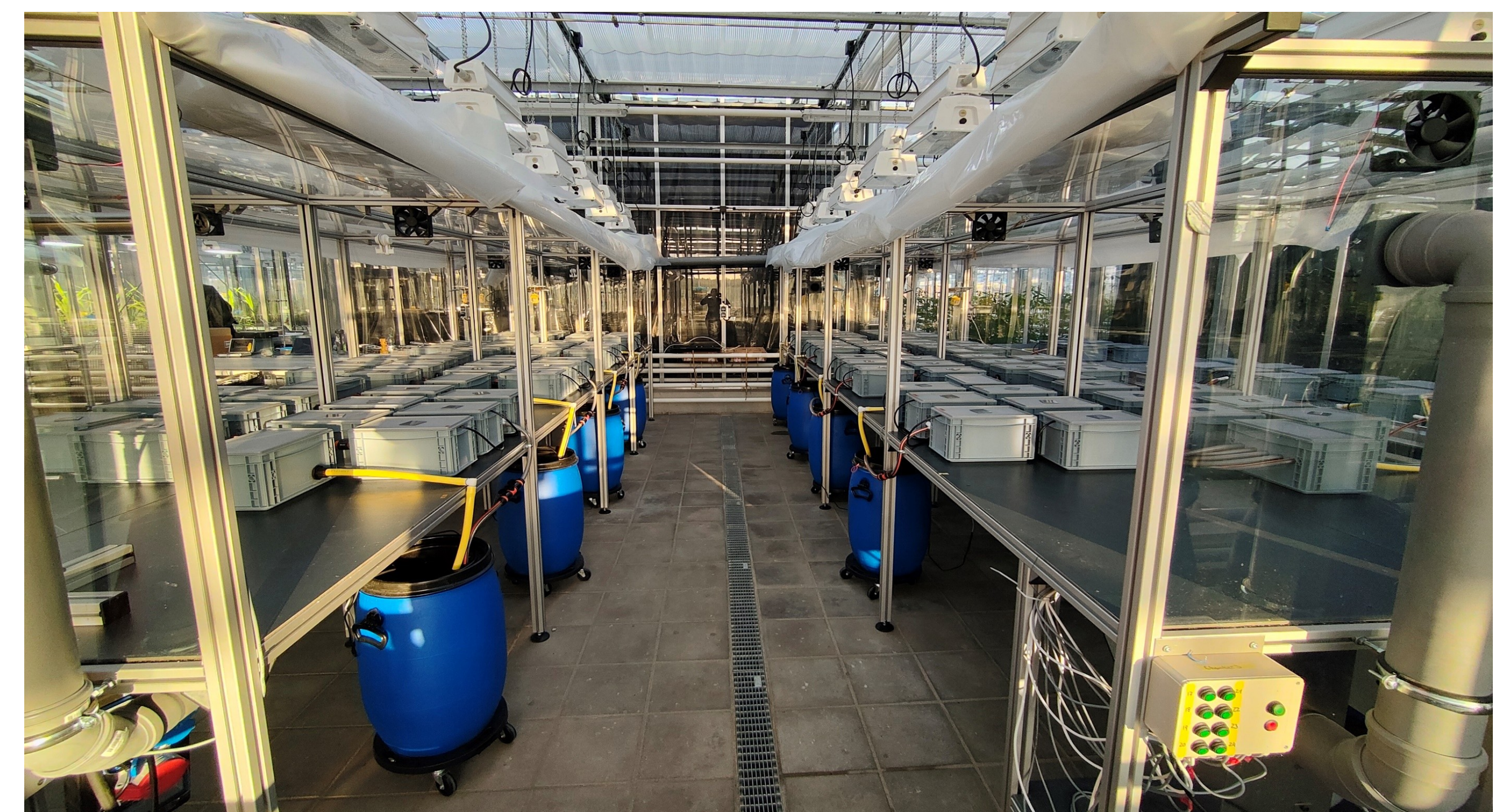
Fig. 1: View of a chamber half with low VPD (left) and a chamber half with high VPD (right) with four hydroponic sets each
