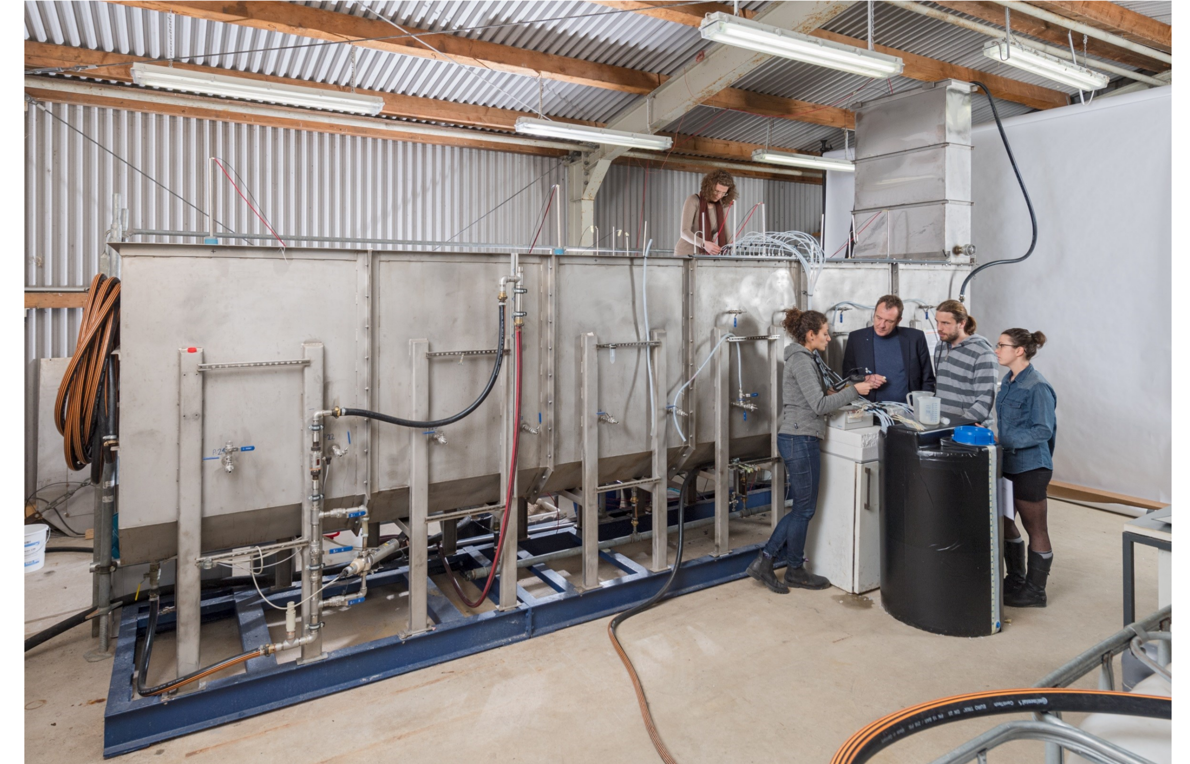
Figure 1: Pilot-scale SMART plus system at the Chair of Urban Water Systems Engineering at the Technical University of Munich, Germany.
