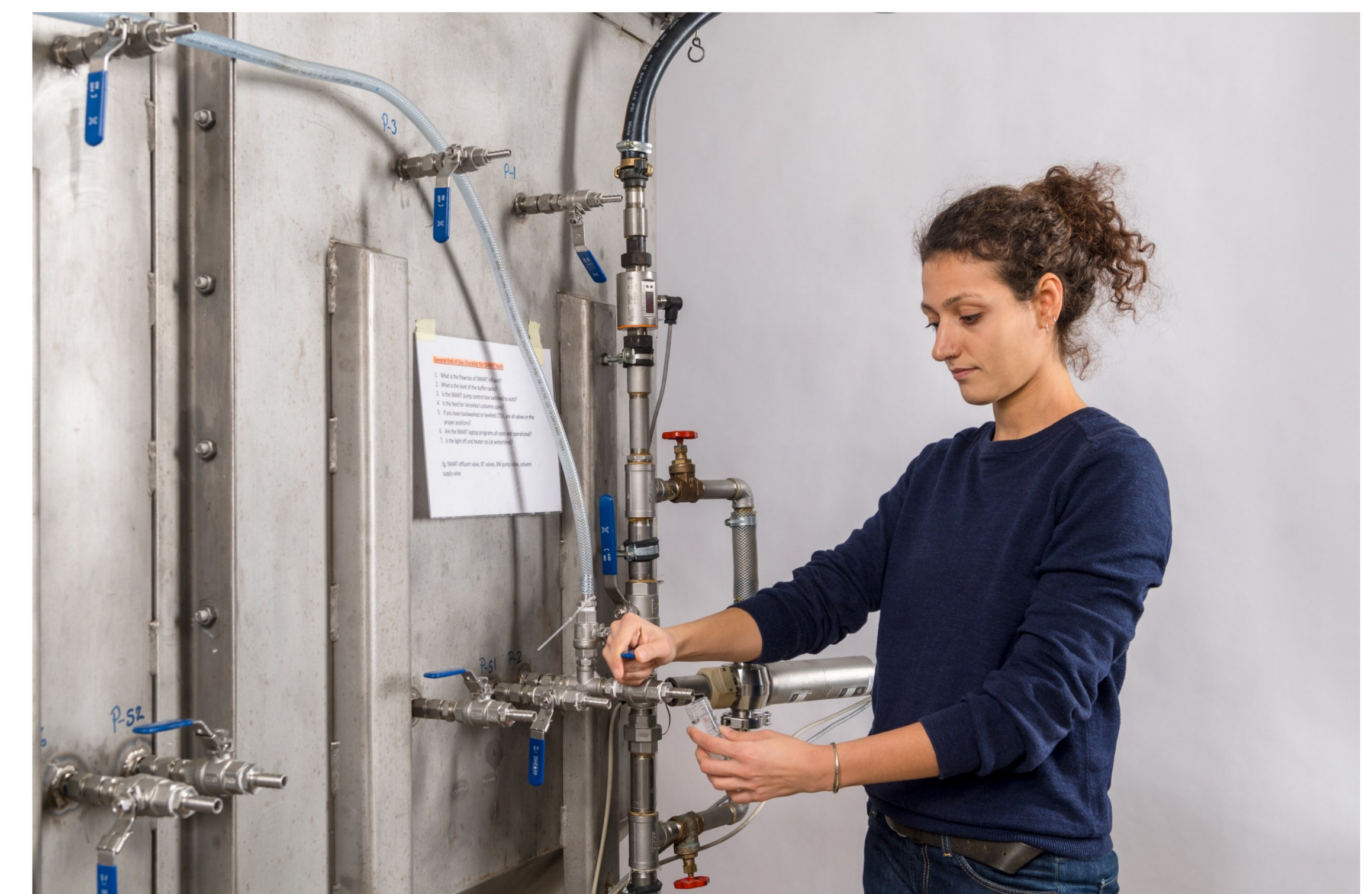
Figure 3: Point sampling and online measurements provide high resolution monitoring of the SMART plus system.
